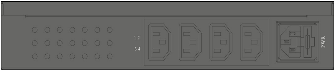
Pic. 4.13 Relay-sensor unit, on the backside
