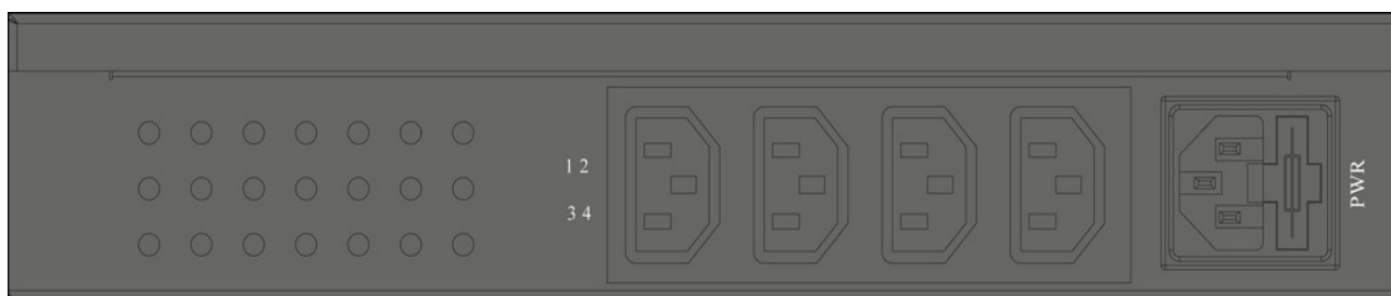
Pic. 3.11 IP Power unit 5505.004, on the backside
