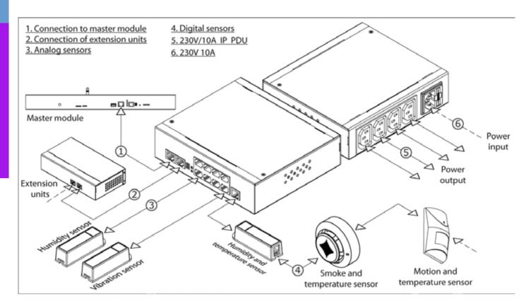
Functions of the system described above can be expanded by connecting additional modules. These modules allow to increase quantity of connected sensors and relay to one system and to increase functioning range. Necessity in such device can arise, for example, in a remote building or office with several floors. Required:
