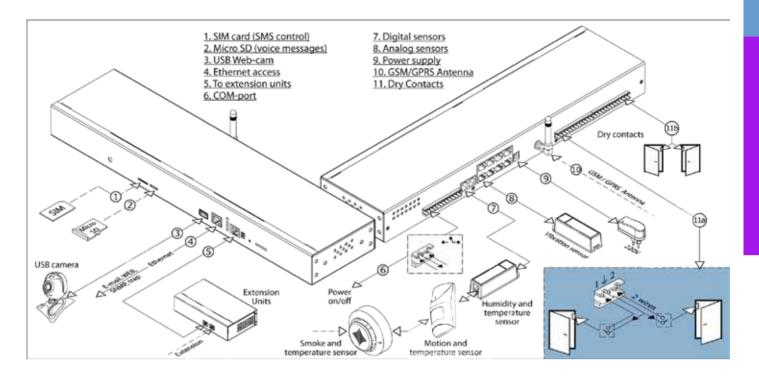
Sensors are connected to master unit's inputs, objects of power supply are connected to the relay, Web-camera is connected to master unit's USB input. Output LAN is connected to any external network, if its not present, LAN is connected to built-in GSM modem.
