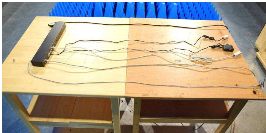
Fig.5: Arrangement of tested sample during the test according to EN 61000-4-3.
