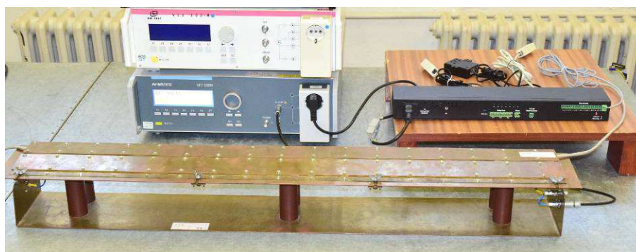
Fig.6: Arrangement of tested sample during the test according to EN 61000-4-4.
