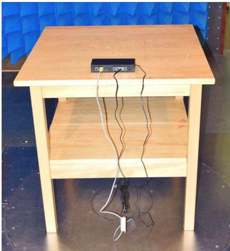
Fig.3: Arrangement of measured sample during radiated emission measurement.
