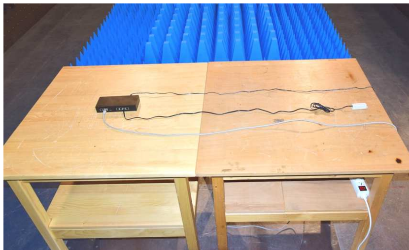
Fig.5: Arrangement of tested sample during the test according to EN 61000-4-3.
