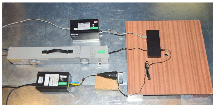
Fig.7: Arrangement of tested sample during the test according to EN 61000-4-6.
