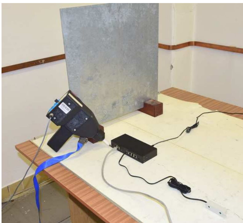
Fig.4: Arrangement of tested sample during the test according to EN 61000-4-2.
