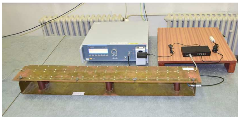
Fig.6: Arrangement of tested sample during the test according to EN 61000-4-4.
